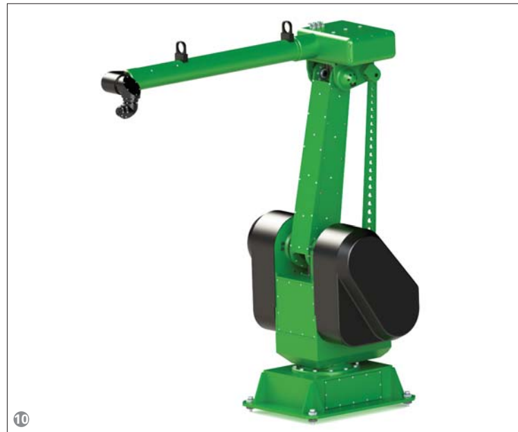
Figure 10: CMA GR 650 ST is a 6-axis robot.
