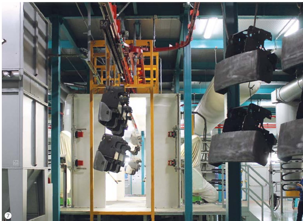
Figure 7: All Gema booths are equipped with the Laser 3D piece recognition device (see the 4 red laser devices at the entrance of the booth).
