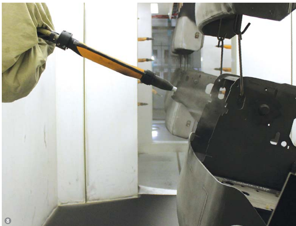
Figure 8: Two of the four CMA opposing robots installed for the automatization of pre touch-up phases.
