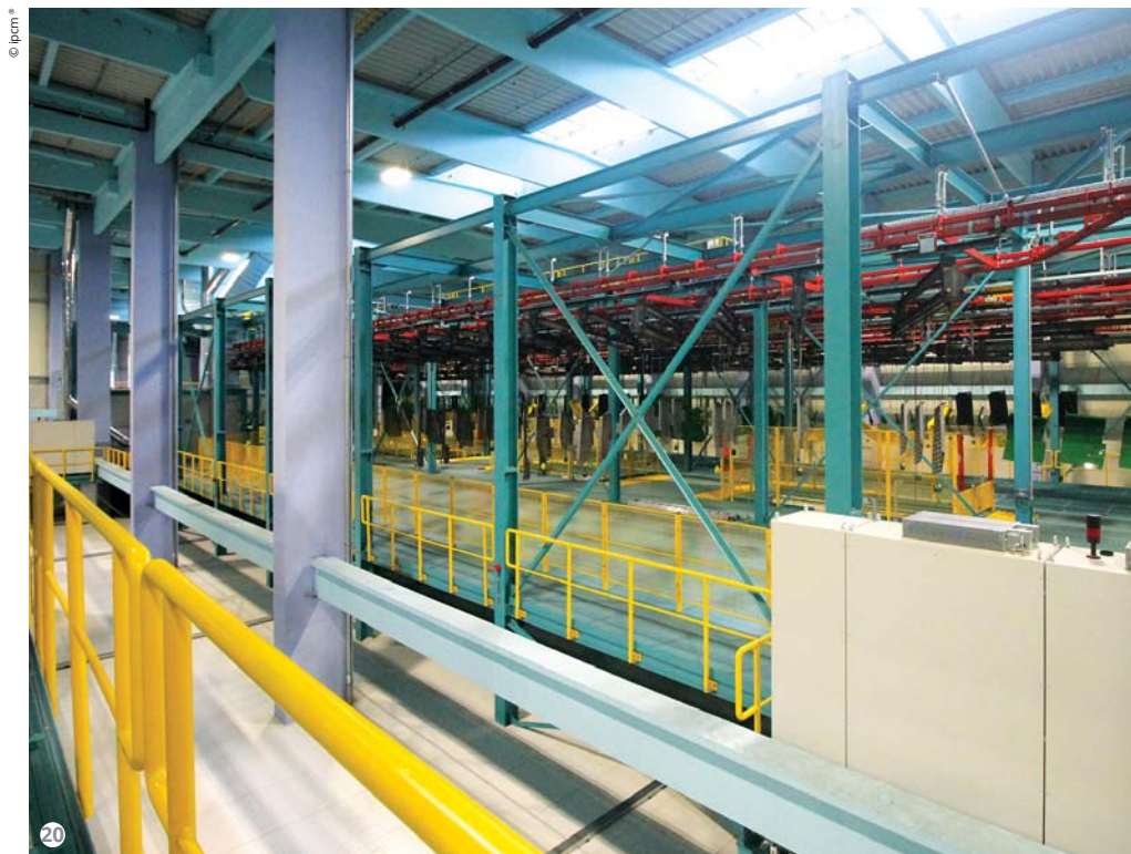
Figure 20: The overhead conveyor with storage buffers of the “plant within the plant”.
