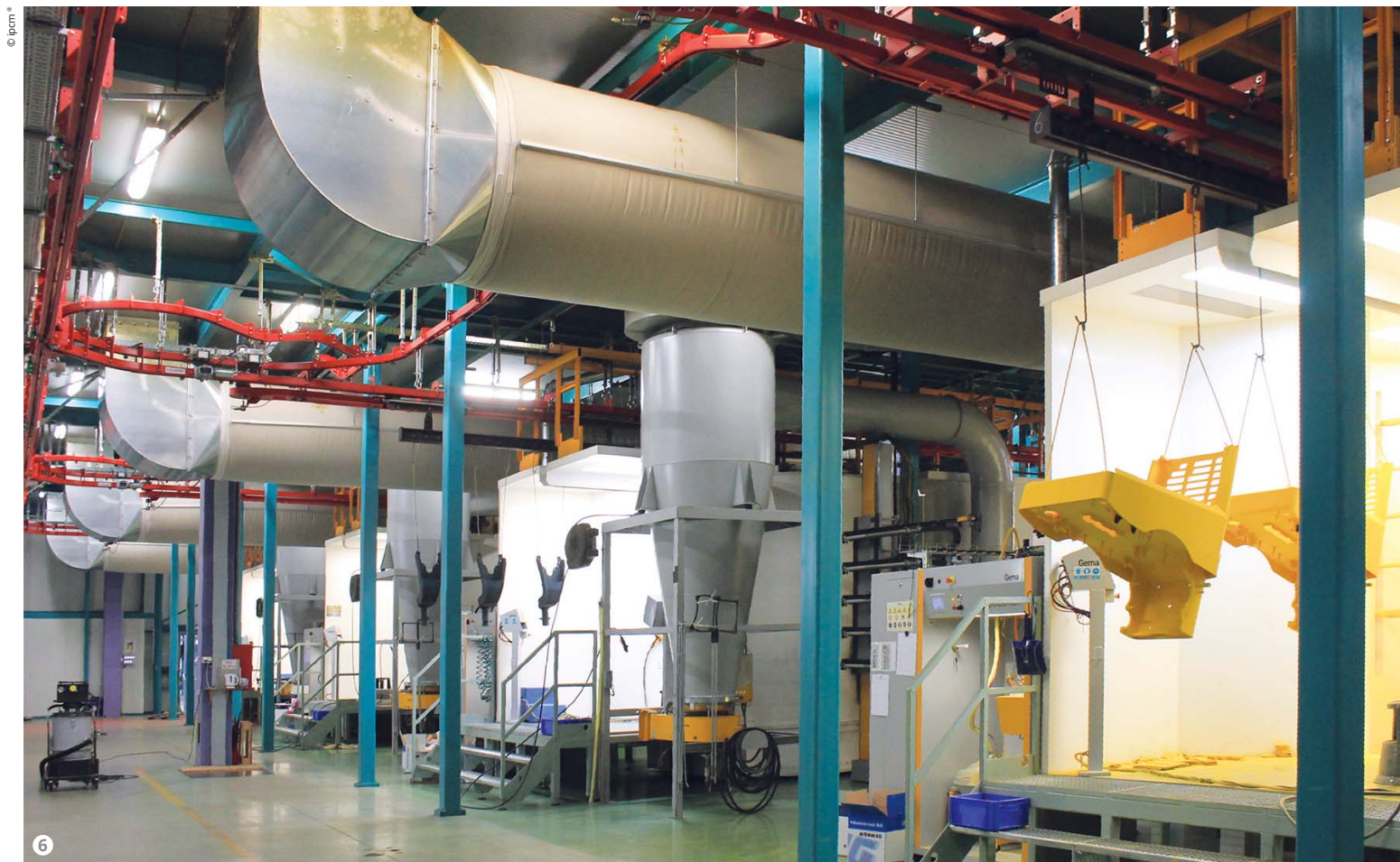
Figure 6: Agrostroj's Painting Line 2 features four Gema automatic coating booths arranged in a dust-free chamber.
