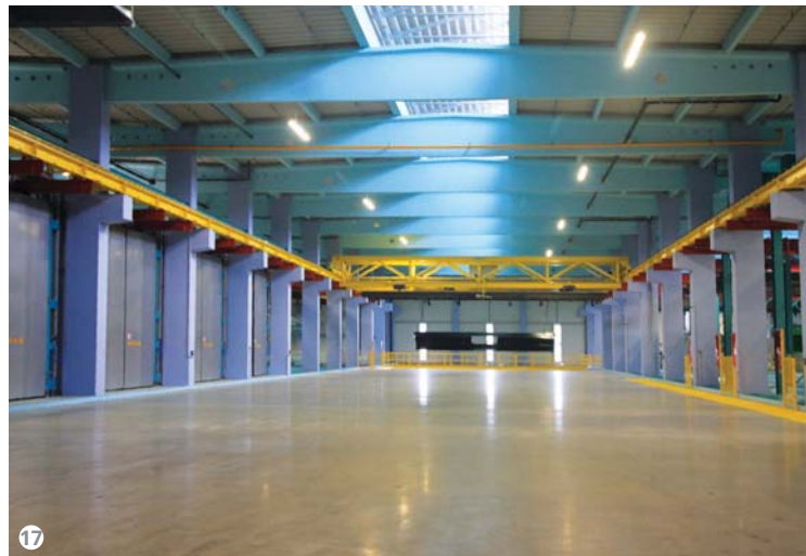
Figure 17: Overview of the six ovens + 6 cooling areas (on the left) and of the powder and liquid coating booths (on the right) located on the upper level of the new huge line
