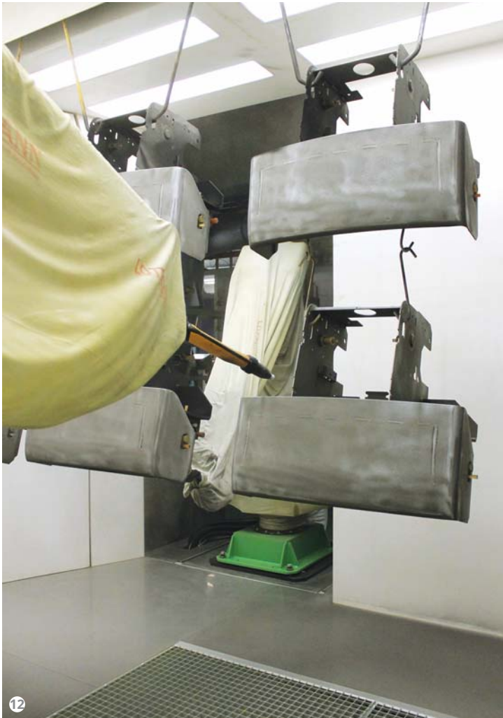
Figure 12: CMA robots are programmed for the coating of 18,000 different automotive parts.
