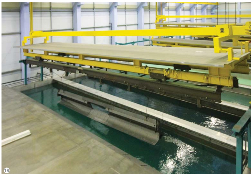
Figure 19: The workpieces are hung onto the flying bars obliquely to promote drainage and avoid bath pollution.
