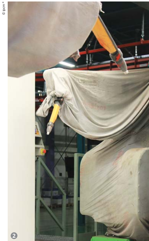
Figure 2: With the installation of four Italian-made pre-retouching robots by CMA Robotics, Agrostroj is the first Central European company to invest in the automation of its agricultural machinery powder coating processes
