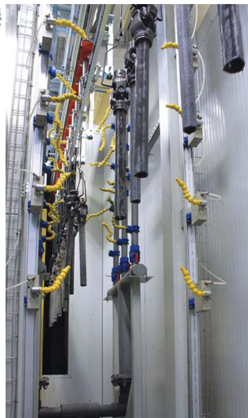
The pre-treatment tunnel and the following blow-off station for the elimination of water residues.
