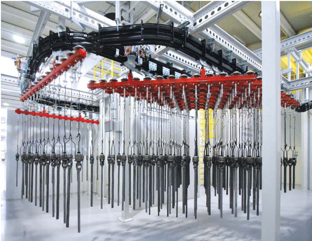
Conveyors Nord's overhead conveyor has a capacity of 600 kg and each load bar is equipped with 14 hooks.
