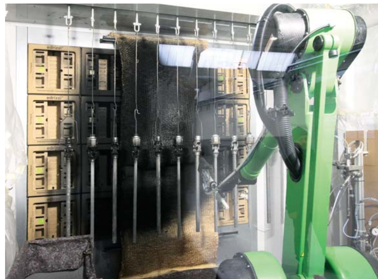
One of the two GR-630 ST 6-axis painting robots supplied by CMA Robotics, equipped with Graco Pro Xpc electrostatic guns.
