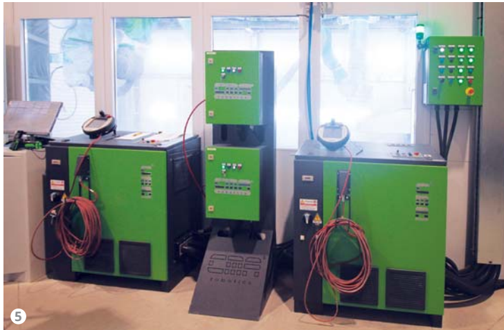
Figure 5: The programming and control devices of the two robots.
