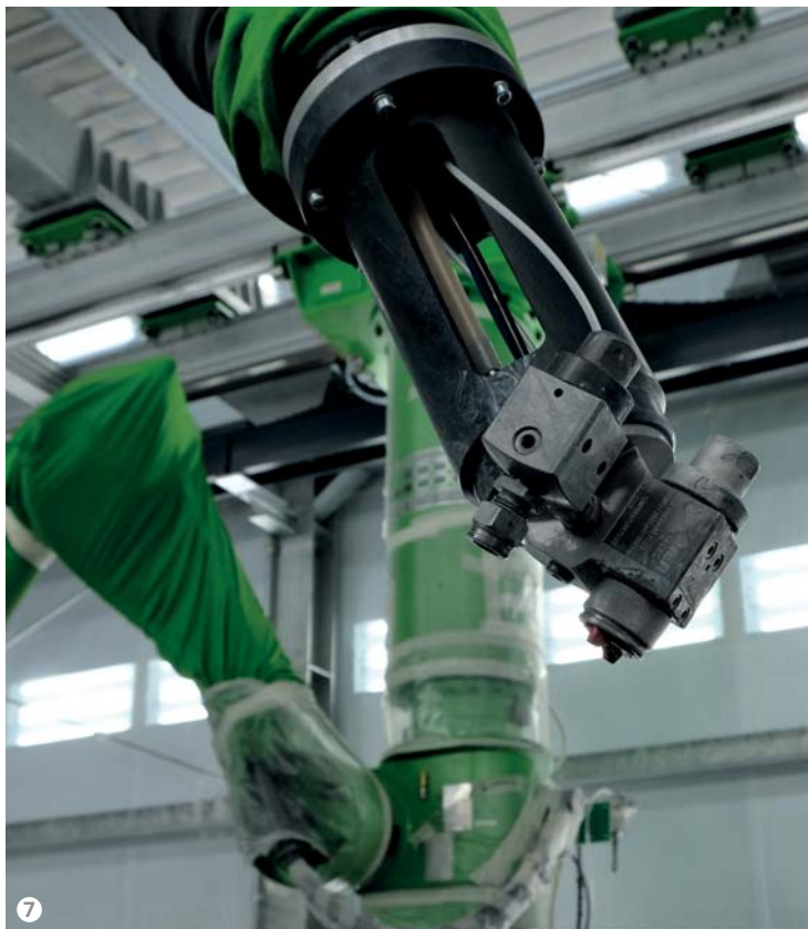
Figure 7: The robots feature Wagner GA 4000 AirCoat automatic guns.
