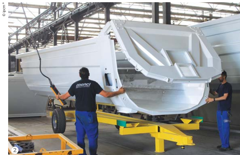
Figure 2: An already-coated tipper taken to the assembly area.
