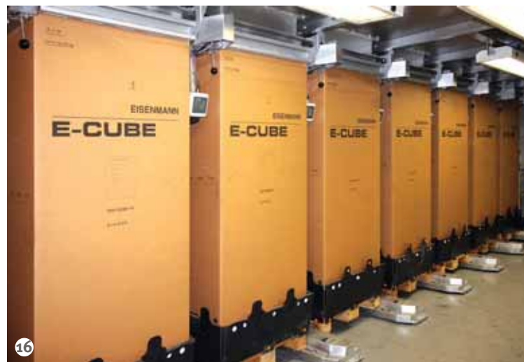
Figure 16: The primer application booth is equipped with Eisenmann’s E-Cube filtration systems.
