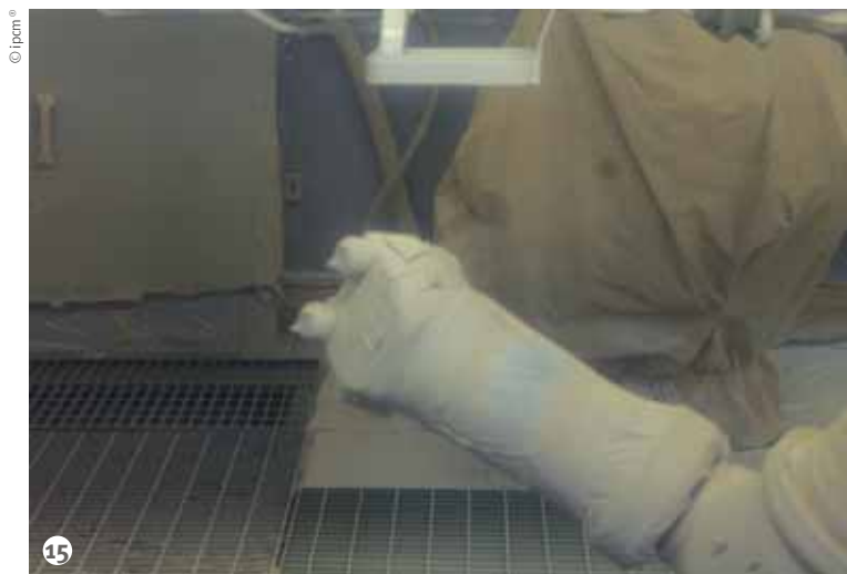
Figure 15: The twin gun technology enables to divide the product volume to be applied between two atomisers.
