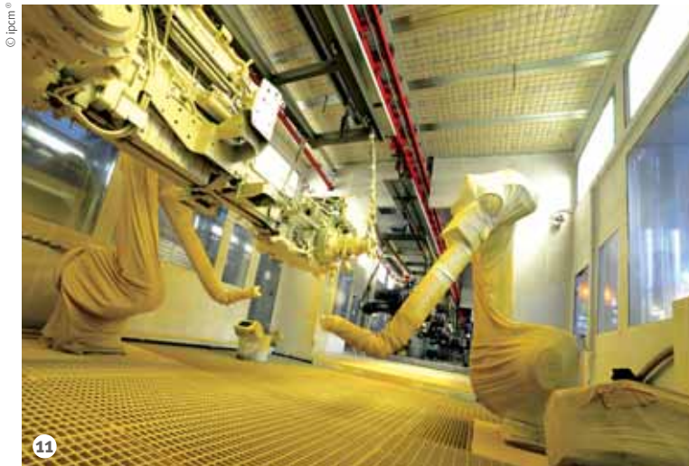
Figure 11: The application of a light coloured primer enables to check that the topcoat layer is applied uniformly.
