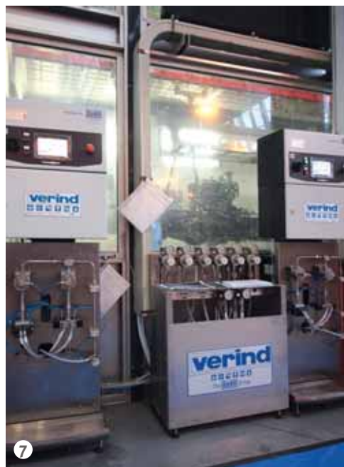
Figure 7: The electronic dosing device EcoDose 2K supplied by Verind.
