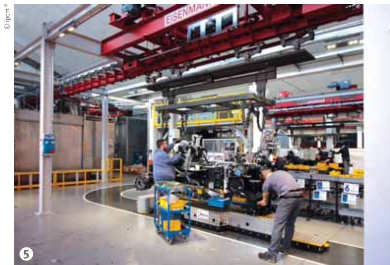
Figure 5: The only remaining manual workstation is the one devoted to masking operations.
